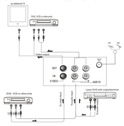
There is also an AV input on the side of your television. Use the Left Audio input (white terminal on the TV), if you are connecting equipment with monosound. The MONOsound will be delivered by both left and right speakers.
